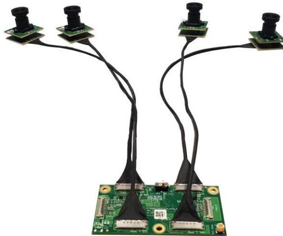
Fig-1: e-CAM130_CUXVR - Four 4 lane MIPI 4K Cameras for NVIDIA Jetson AGX Xavier
